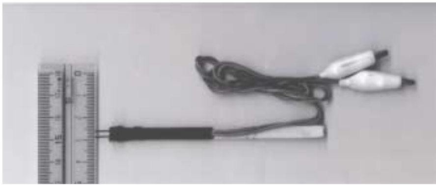
Fig.2: The electrodes for measurement of electric conductivity
